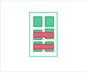
When use 6pin socket and use the +5V in 6pin socket to power this level board
